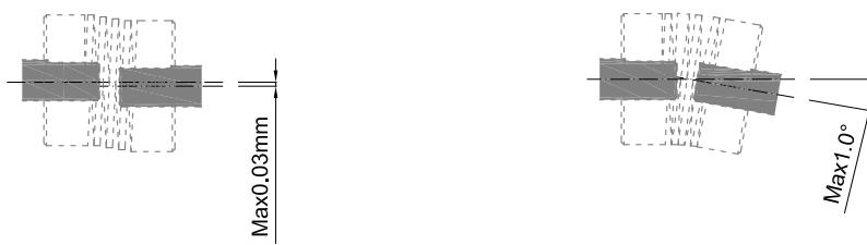
Notice : coaxiality between shaft of encoder and power shaft must be less than 0.03mm, and gradient must be less than 1.0°.
